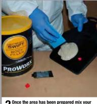
Once the area has been prepared mix your ProWorx filler with hardener at a ratio of 2% at an ambient temp of 20°C.
