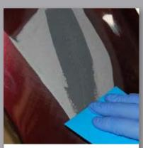
**9** Take the applicator supplied and spread the Plex smoothly on the outer repair surface.
