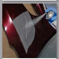
**6** Degrease both sides and apply a thin layer or coating of adhesion promoter.
