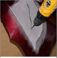
**3** Drill a hole approximately 3mm at the end of the split to relieve the chance of further cracking/splitting.
