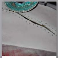
4 Drill a number of 3mm holes either side of the repair (this is known as shoe lacing). Then using a die grinder/file grind a "V" shaped channel into the repaired area. Key the back of the plastic in the area to be repaired.
