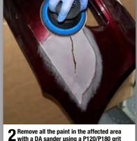
**2** Remove all the paint in the affected area with a DA sander using a P120/P180 grit
