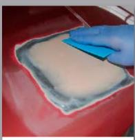
Apply your full coat of filler with the applicator provided making sure that firm and even pressure is being applied.
