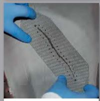
**5** Take a piece of fabric webbing material and cut to the approximate size of the repair.
