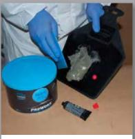
**4** Once the area has been prepared, mix your FibreFix filler with hardener at a ratio of 3% at an ambient temp of 20°C.
