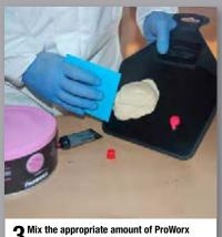
**3** Mix the appropriate amount of ProWorx finishing filler at a ratio of 2% at an ambient temperature of 20°C.
