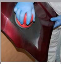
$10^{\,\text{Once cured, apply dry powder guide}}_{\,\text{coat.}}$
