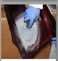
**1** Block sand with either a P120 or a P180 feathering out with a P320 to finish.
