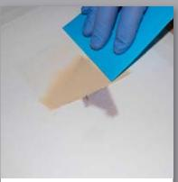
**8** Then apply a full coat of ProWorx bulk filler with the applicator provided making sure that firm and even pressure is being applied.
