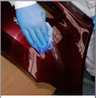
Clean and degrease the area to be repaired on the front and reverse.
