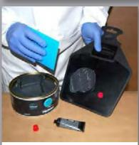
**7** Mix the appropriate amount of Plex filler with hardener at a ratio of 2% at an ambient temp of 20°C.
